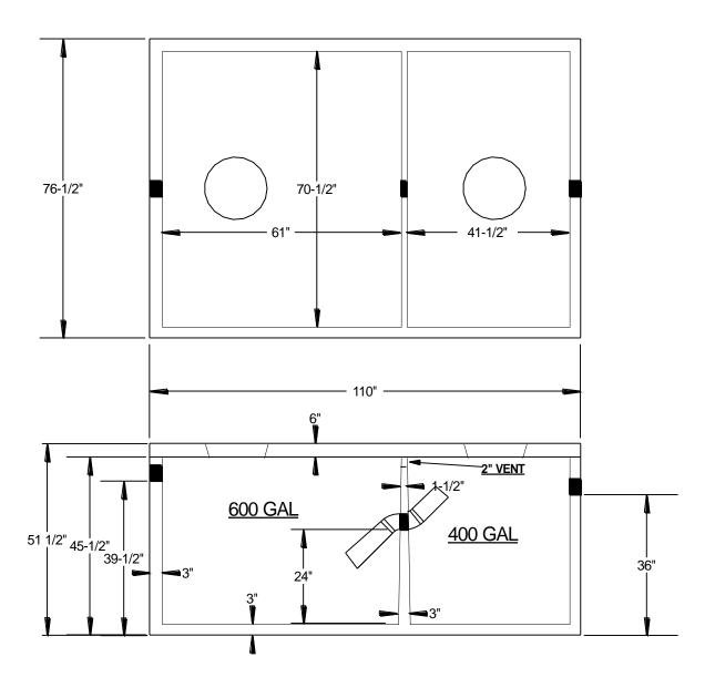
CLASS 1 CONCRETE WITH DESIGN STRENGTH OF 4500#PSI IN 28 DAYS. UNIT IS OF MONOLITHIC CONSTRUCTION AT FLOOR TO REQUIRED DEPTH ON TANK.
